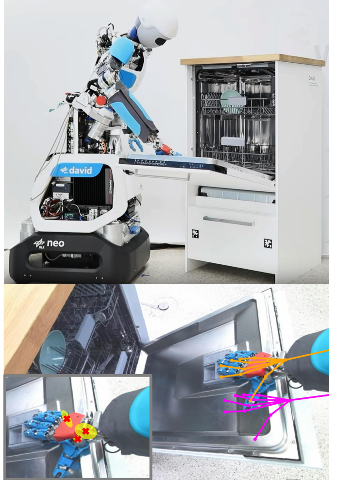
Fig. 1. The humanoid robot neoDavid empties a dishwasher. In the bottom image, the error of the forward kinematics (magenta) of the robotic arm can be clearly seen, motivating a vision supported pose estimation (orange). The vision input is our PK-ROKED algorithm, which provides the image location and the associated covariance of selected keypoints (shown red and yellow in the insert, bottom left) for a subsequent sensor fusion. Image: ©DLR.
