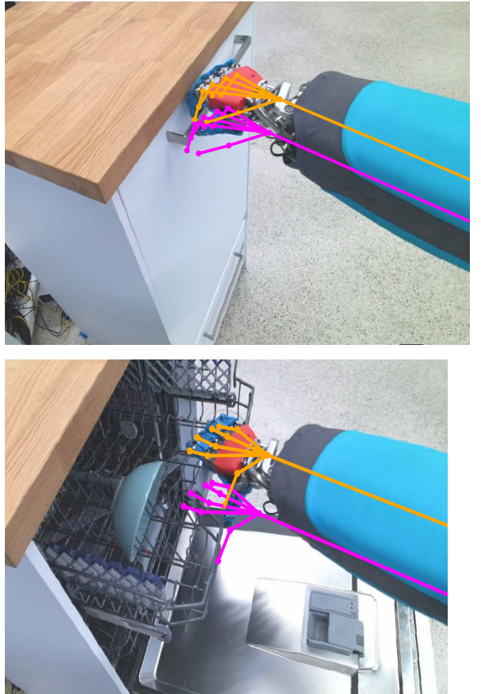
Fig. 12. Evaluation of our fusion results on the neoDavid data, while the robot empties a dishwasher. The pose estimation of our approach is highlighted with the orange skeleton. Whereas, the forward kinematics are shown in magenta. As one observes, our approach is able to significantly improve the pose estimation.
