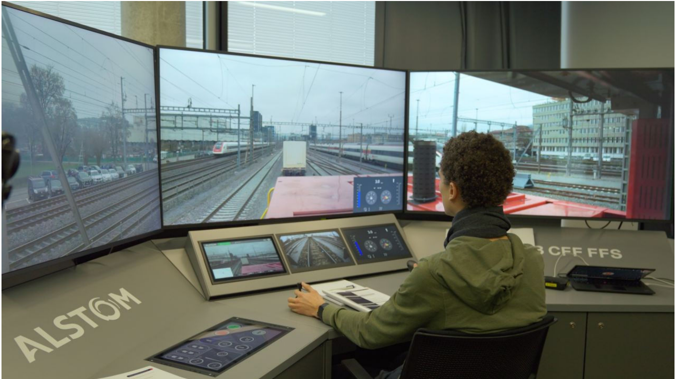
Figure 2. Prototype of a remote locomotive control system tested in the field. The controlled locomotive Aem 940 was located in the Mülligen shunting yard. The RO was located in an office building in Oerlikon.
