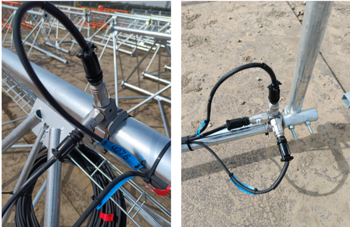
Figure 2: Instrumentation of the sensors on the ground at the construction site. Left: biaxial measurement point on a mast segment. Right: triaxial measurement point at the end of a boom tube.
