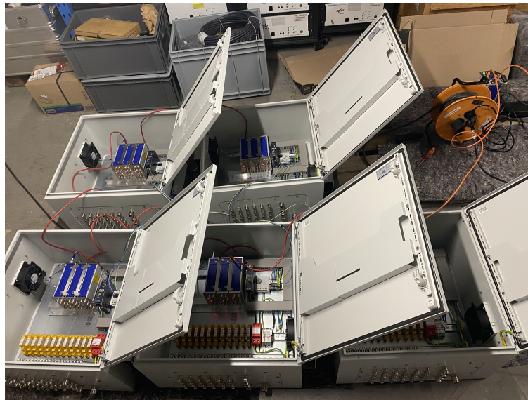
Figure 4: Final check of control cabinets before the installation. The measuring modules are connected to each other with a patch cable.
