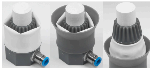
Fig. 3. Rolling-lobe isolator assembled and depressurized. From left to right: without external guide, with external guide, piston extended.
