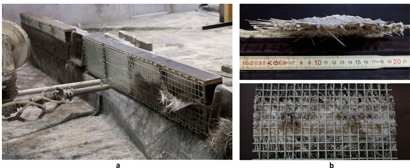
Fig. 6 a Concurrent spraying of short glass fibres and concrete on fibre meshes; b Formation of a separation layer of short fibres visible in sectional image (top) and in rear view (bottom)
