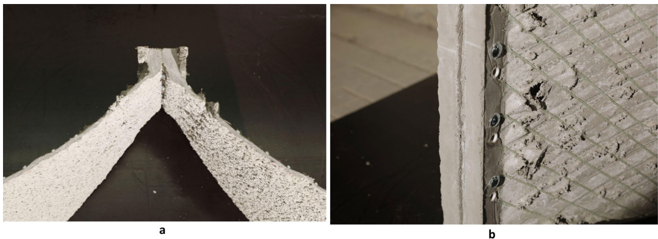
Fig. 20 Testing the joining principle on two cut-outs from the demonstrator: a Sectional view; b Detailed view of bolts
