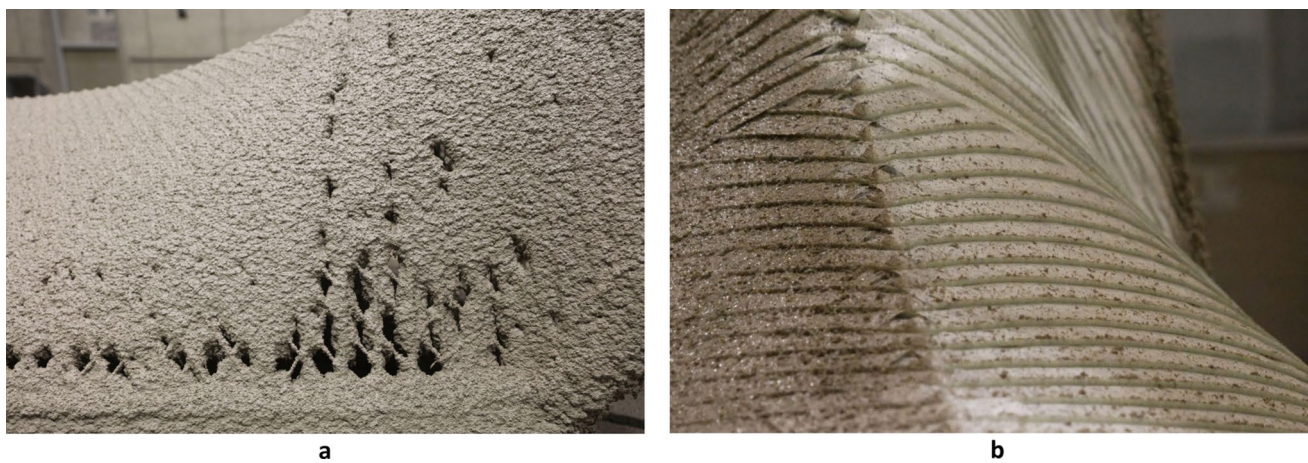
Fig. 17 a Holes formed during RASP process as seen on the top side; b Visible aggregate separation
