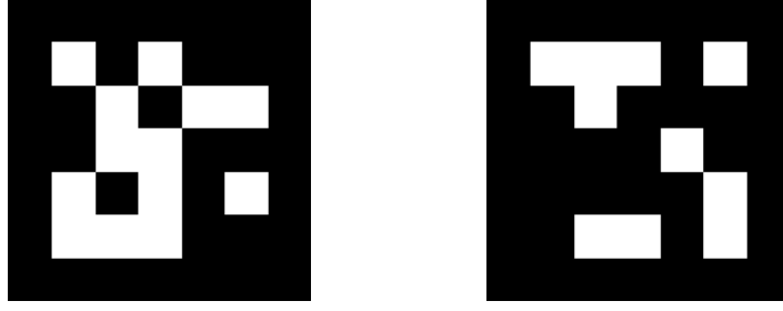
Figure 7: Exemplary ArUco markers with ID 0 (left) and ID 5 (right) [18].
