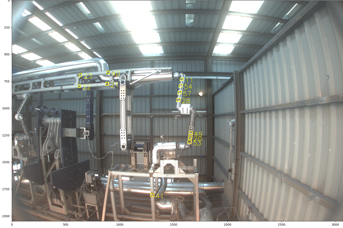
Figure 14: Exemplary image of camera A with the detected markers and their unique IDs. Here, not all markers were detected along the lower tube.
