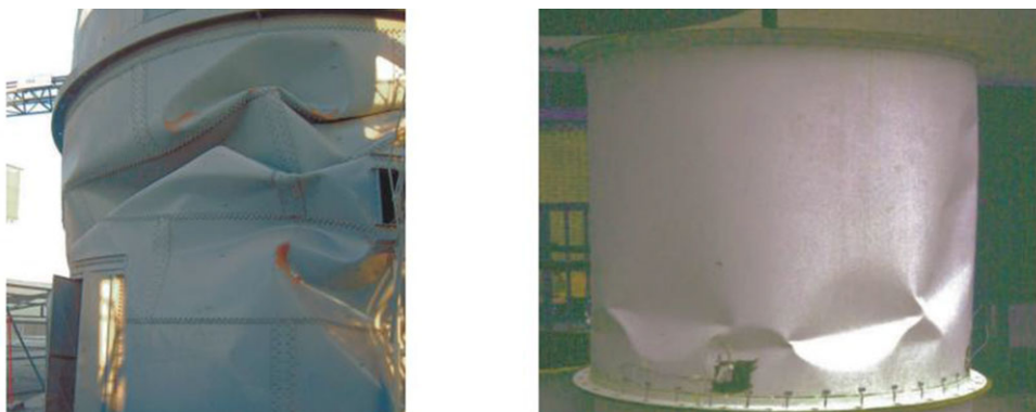
Figure 1. Cylindrical shells under axial compression: failure in service (left), laboratory test (right) from [2].
