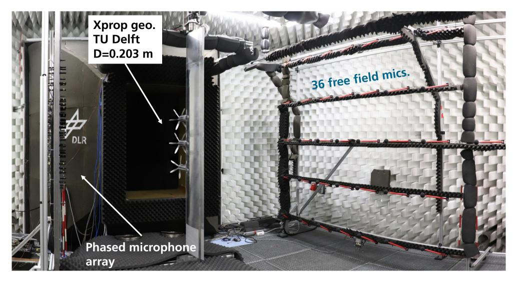
degrees of freedom: stagger, rotation direction, phase, AOA, prop spacing, advance ratio, wing flap angle
