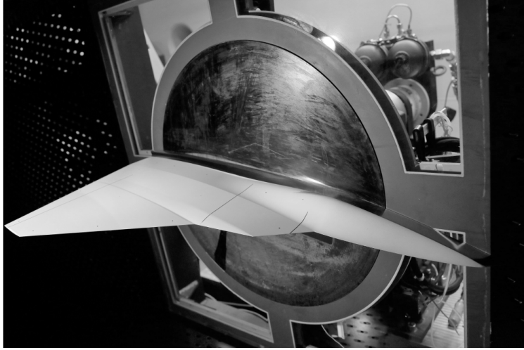
Fig. 3 Image of the DLR-F23 test model installed via its peniche in the test section of the DNW-TWG wind tunnel.
