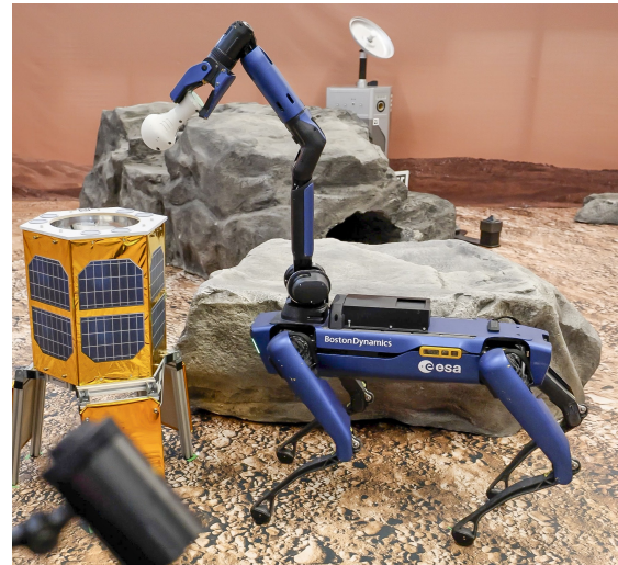
Fig. 3: ESA's integrated Spot robot dropping a sample in the handover station.
