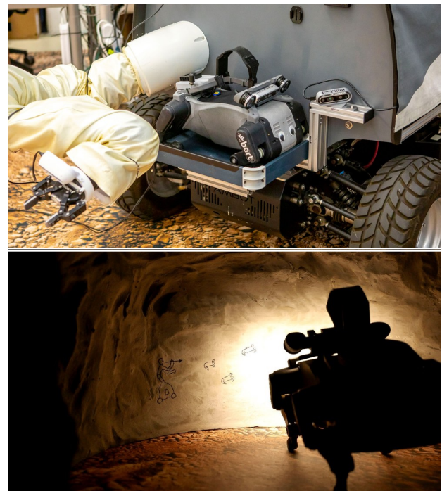
Fig. 4: The small-sized quadruped Bert during the Surface Avatar mission being transported by ESA's Interact rover (top) and during the exploration of a cave (bottom).
