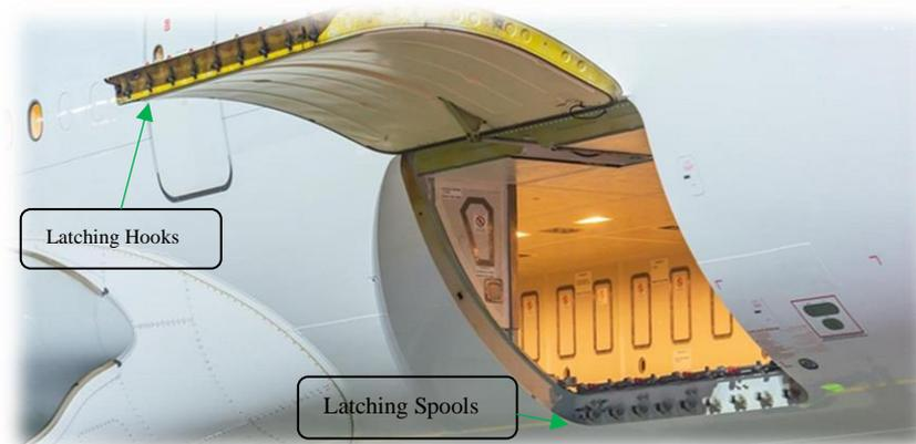
*Figure 1-1 Main deck cargo door of an Airbus A320-neo aircraft [1]*
