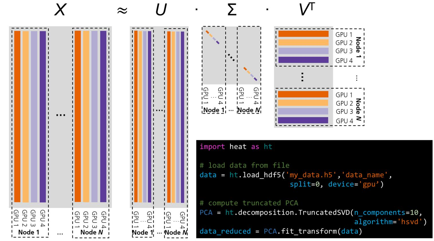
Illustration of the planned functionality: a simple scikit-learn-like API allows to compute the SVD of a huge matrix using several nodes of a GPU-cluster.
