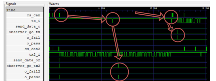
Figure 6. Traces for a CAN IP transmission process where the data transmitted by cs_can2 trojanises cs_can in order to start an un-acknowledged sending process (tx_i).
