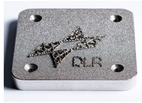
Fig. 1 View of the flight sample built during the MAPHEUS-10 sounding rocket flight. The thickness of the sample is limited to eight-layers due to the available microgravity time of 6.5 min. The build is completely welded to the platform without detaching. The sample thickness mildly decreases toward the right half, due to feed-stock particle transport coming in from the left
