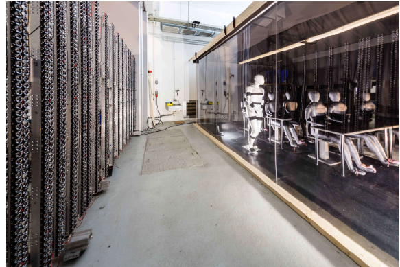
Figure 1: Research seminar room with transparent walls and ceiling at DLR Göttingen for investigations of mixed turbulent convection flows using several seated and one upright and traversable thermal dummies. 3D Lagrangian Particle Tracking with Shake-The-Box will be used to track millions of submillimeter Helium-Filled-Soap-Bubbles (HFSB) illuminated by a large pulsed LED array.
