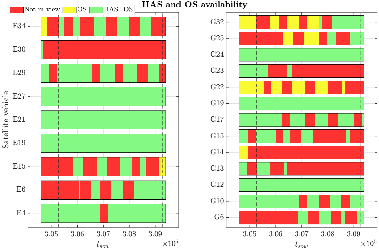
Figure 8.8: HAS IDD and OS corrections availability during the experimental campaign. Dashed lines indicate take off and landing epochs, respectively.
