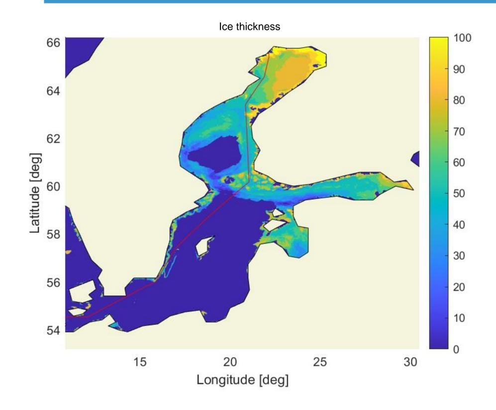
The conceptualized research vessel for maritime energy systems developed by DLR is used as subject for the demonstration case. It will occasionally operate in ice, e.g. along an exemplary route from Kiel, Germany to Lulea, Sweden. Typical ice conditions on this route are derived from Weibull fit Copernicus data.
