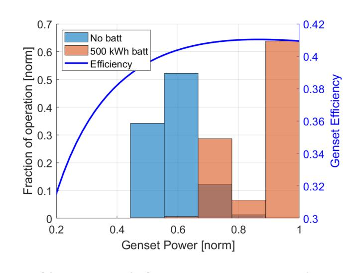
Use of batteries shifts operation points during winter voyage with ice conditions to higher efficiencies
