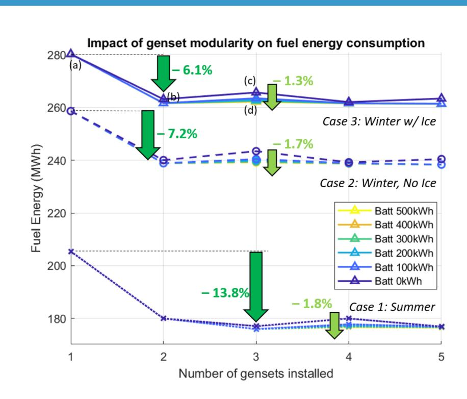
Hybridization and modularization of the energy system increases the overall energy efficiency.
