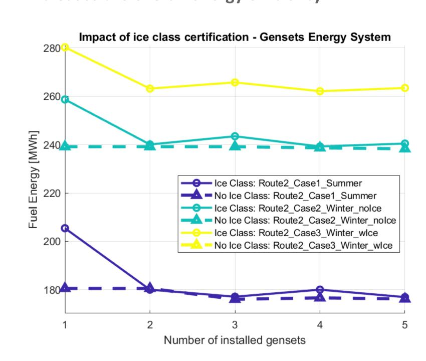
The efficiency increases significantly if the energy system of an ice class vessel is modularized.
