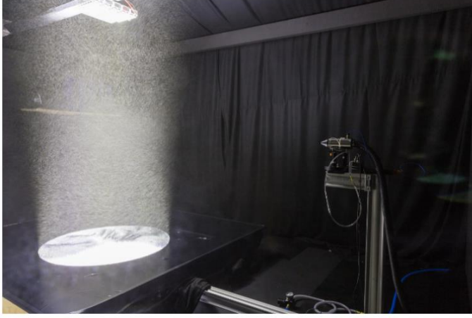
Figure 1: Experimental setup. Left: 82 \text{ m}^3 test room with LED arrays illuminating the test section, the cylindrical STB measurement volume and a d = 10 \text{ mm} nozzle. Right: top view of calibrated camera system, showing the common illuminated volume of \sim 1.85 \text{ m}^3
