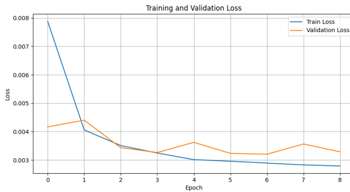
Figure 4.2: Training and validation loss curves during fine-tuning of DINOv2. Early stopping is triggered after the 9th epoch when validation loss no longer improves.
