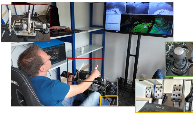
Fig. 3. Control station used for teleoperating a remote mobile robot. Credit: DLR (CC BY-NC-ND 3.0)
