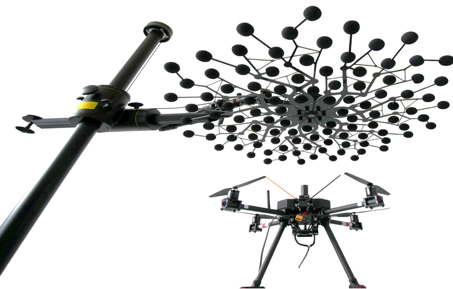
Fig. 3: The acoustic camera is mounted above the UAS, which is in parking position on ground level.
