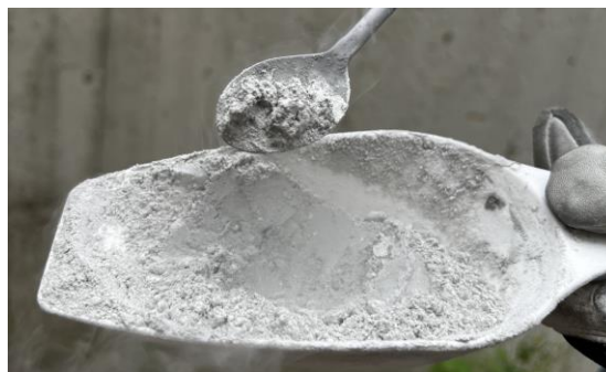
Figure 5: Icy regolith simulant after finishing the mixing of dried regolith simulant with ice particles.
