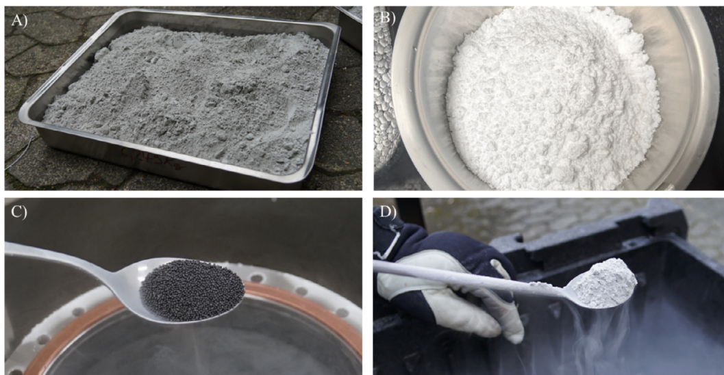
Fig. 3. Simulants used in the LUWEX project. A) LUNEX Regolith simulant, B) Ice particles, C) Glass beads, and D) the mixed Icy Regolith simulant.
