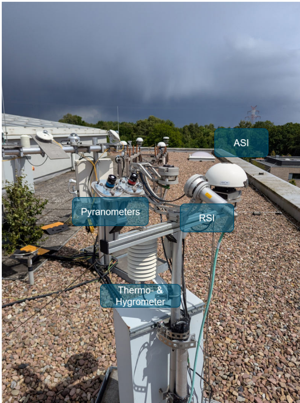
Figure 2: Typical setup of Eye2Sky station (station OLUOL) with all-sky imager (ASI), rotating shadowband irradiometer (RSI) and additional meteorological sensors.
