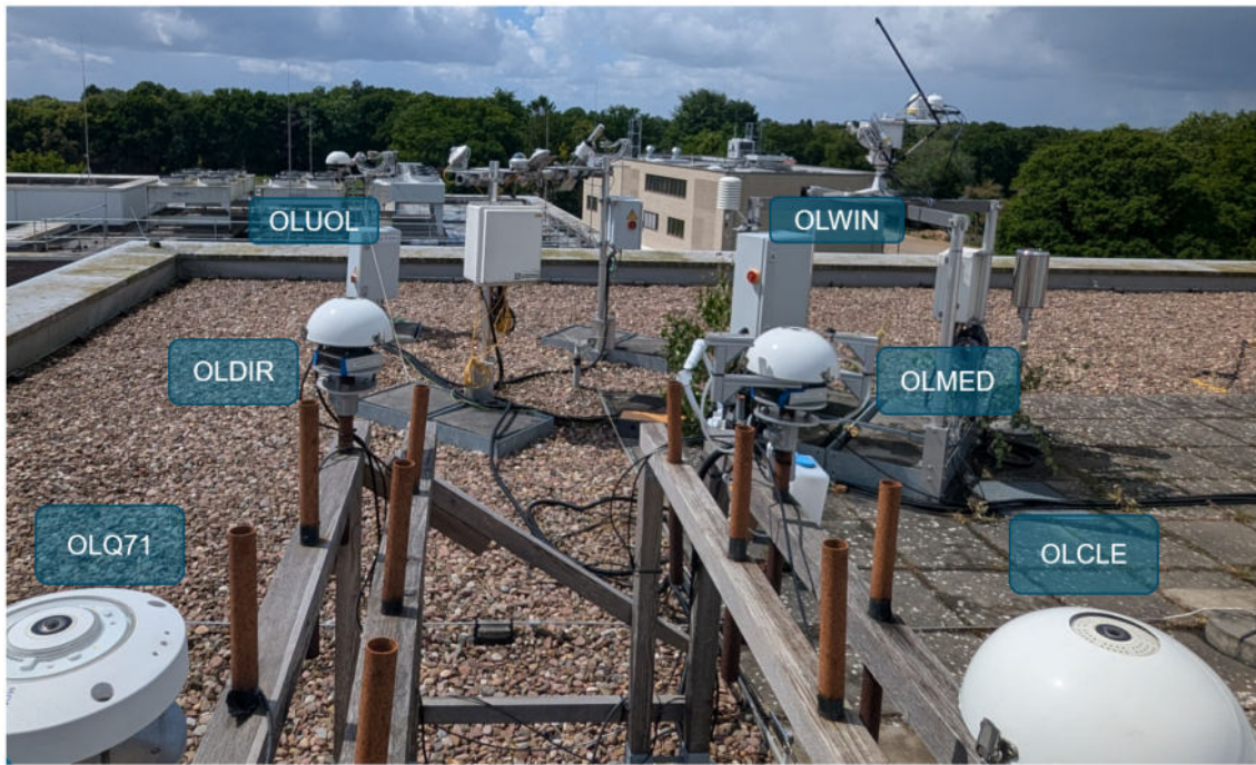
Figure 10: Experimental setup of this study on rooftop of building W33, stations equipped with all-sky imagers (ASIs) (OLCLE, OLDIR, OLMED, OLQ71, OLUOL), and meteorological reference station (OLWIN).
