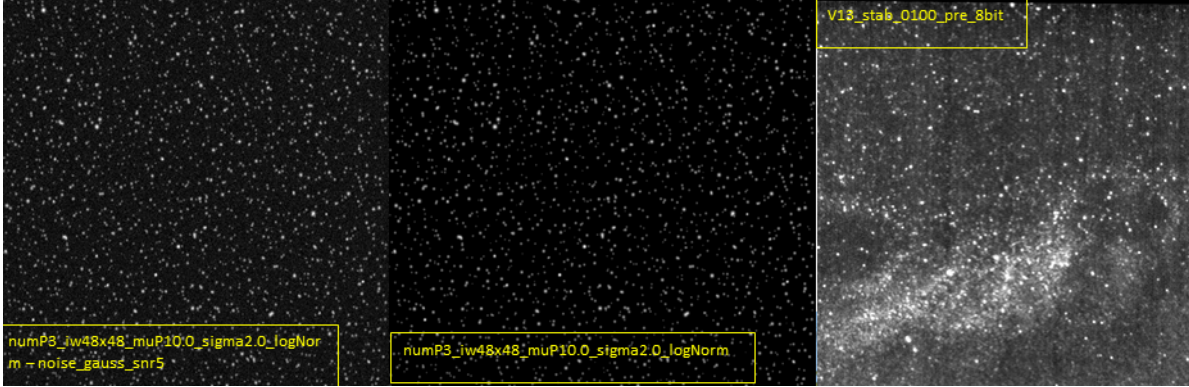
Figure 7.60: synPIV synthetic raw particle image comparison. Two on the left from synPIV, right image from experimental first H2K campaign (Run1007).
