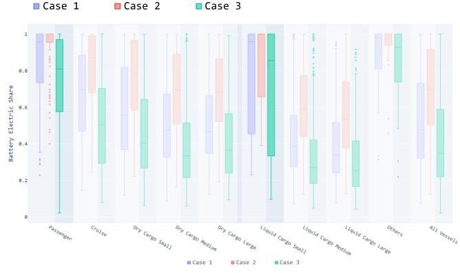
→ Hybrid Propulsion Systems could reduce tank-to-wake CO<sub>2</sub> emissions by 26 – 52%
