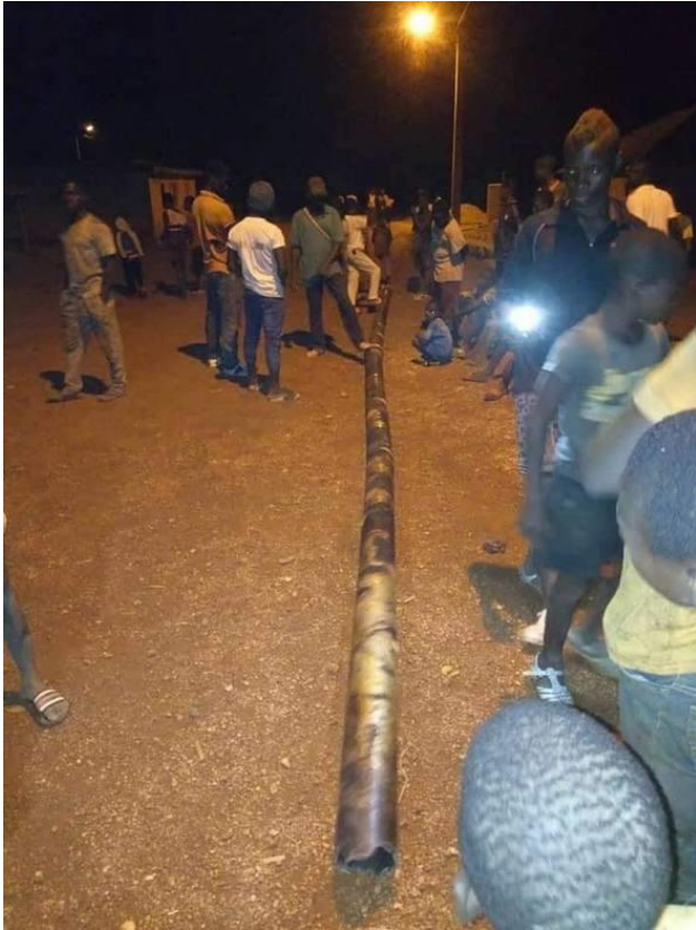
Figure 9: Discovered debris associated with CZ-5B Rocket Body (NORAD ID 45601) [10]
