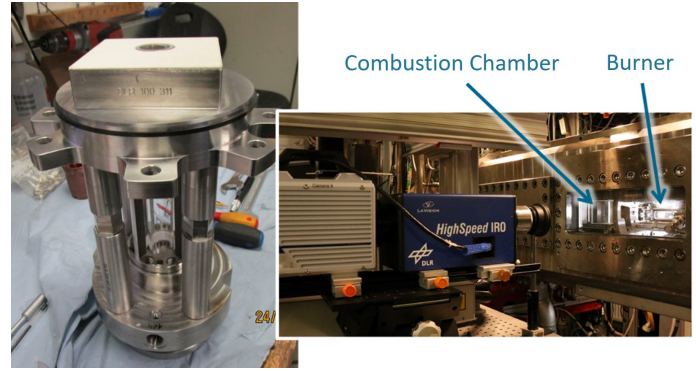
FIGURE 3: Optical mixing duct. Left: single nozzle with quartz glass mixing duct before mounting to combustion chamber; right: setup of high-speed OH* CL for flashback observation in the optical mixing duct.
