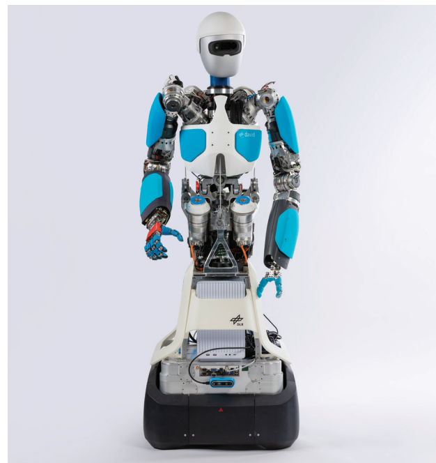
FIGURE 1. The dexterous humanoid neoDavid is assembled of the elastic upper body David and the four-wheeled omnidirectional mobile platform NEO.
