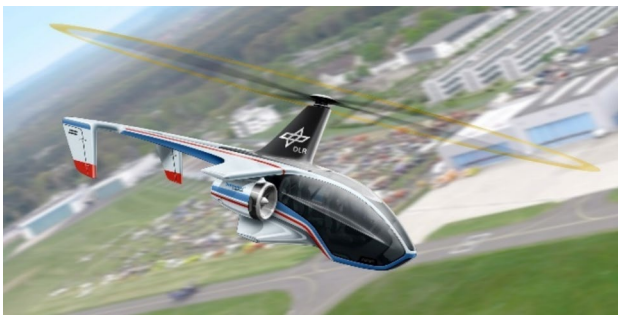
Fig. 3 S 2 TOL gyroplane variant 2 with ducted propellers
