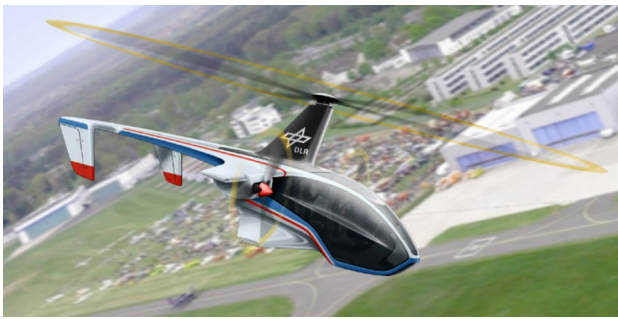
Fig. 2 S 2 TOL gyroplane variant 1 with conventional propellers
