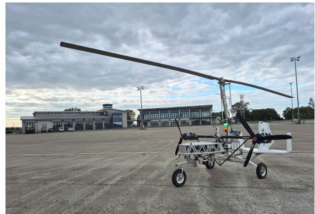
Fig. 15 Demonstrator#1 with electrically driven propellers (380 kg MTOM)
