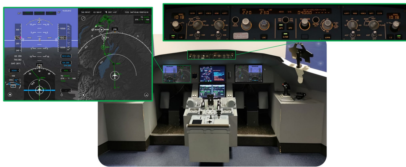
Fig. 7 Flight test simulation bench (Thales, Toulouse) with new generation Cockpit Display System (upper left, comprising ND and PFD) and A320 family Flight Control Unit (upper right)
