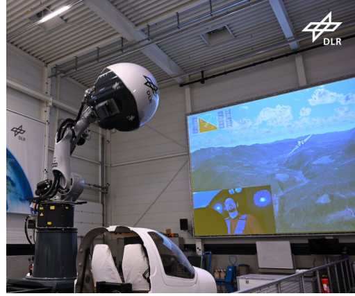
Figure 1.2. Robotic Motion Simulator (RMS) at the German Aerospace Center [19]
