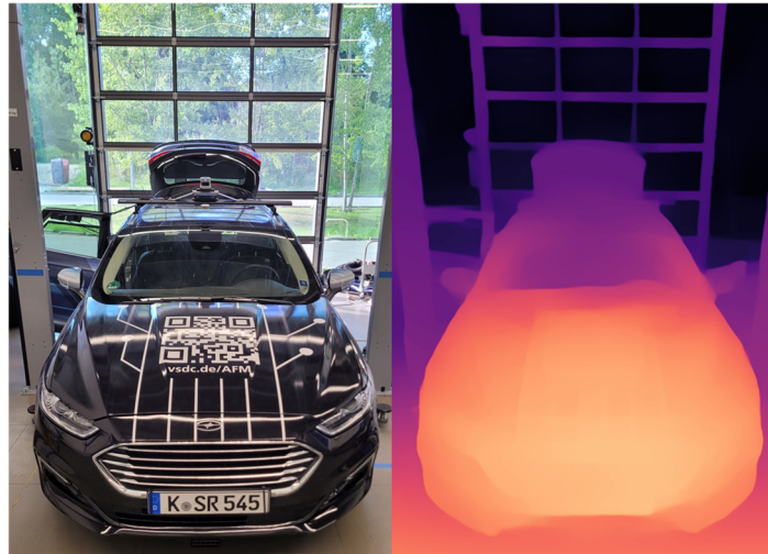
Figure 10. Depth image of the AFM research vehicle generated by MiDaS. Light areas represent nearby objects, dark ones represent more distant objects.
