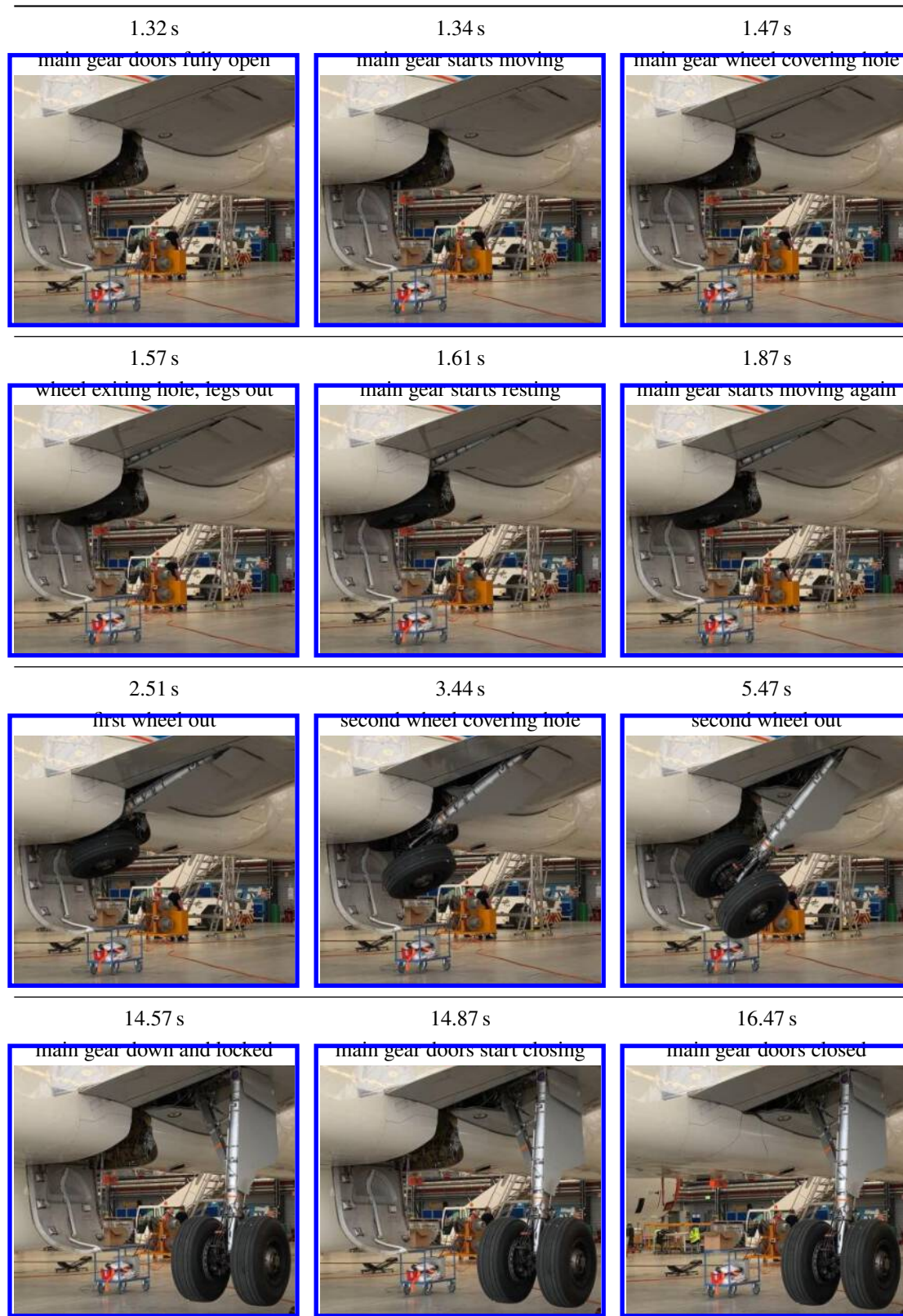
Fig. 5 Key frames for the main gear extension motion extracted from the Airbus A320 ATRA maintenance video; credits DLR (CC BY-NC-ND 3.0)
