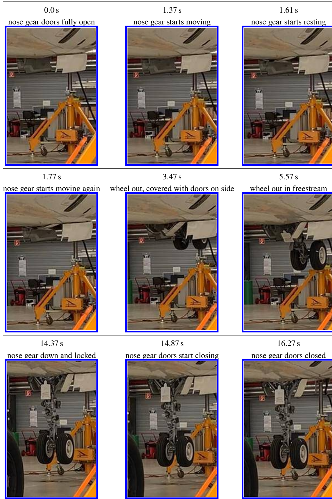
Fig. 4 Key frames for the nose gear extension motion extracted from the Airbus A320 ATRA maintenance video; credits DLR (CC BY-NC-ND 3.0)
