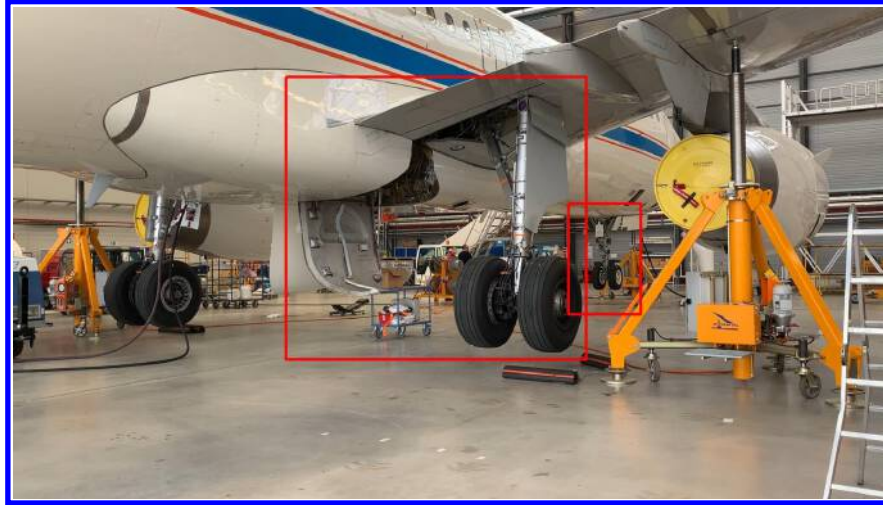
Fig. 3 Full frame from DLR's Airbus A320 ATRA maintenance video with red rectangles indicating the areas of interest for the gear extension sequence analysis, cf. Figs. 4 to 5.
