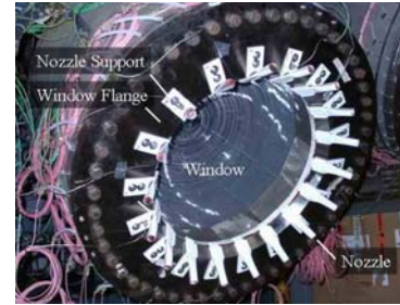
Fig. 30: Preinstalled nozzles on window flange of high-temperature receiver
