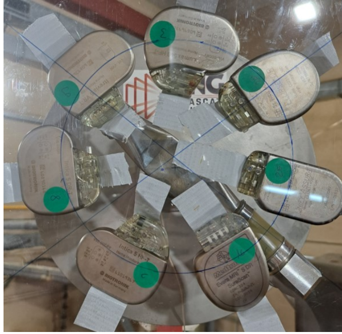
Figure 6.2: Set up of CIEDs at FNG at a radius of 8 cm at 5 cm distance to the target which is behind the acrylic glass plate in this picture.
