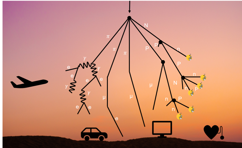
Figure 2.2: Cosmic radiation shower in the atmosphere showing neutrons (n), protons (P), pions ( \pi ), muons ( \mu ), electrons (e), gamma-photons ( \gamma ) and other nuclei (N), adapted from (Baumann and Kruckmeyer, 2019).
