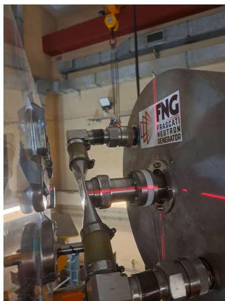
Figure 4.9: Set up of the medical devices in front of the tritium target of the FNG.
