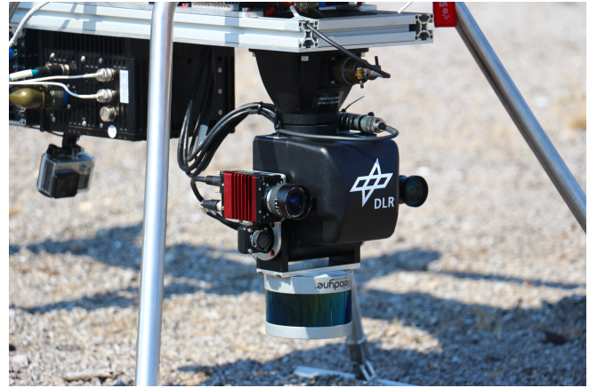
Figure 1: Experimental sensor setup mounted to the payload bracket of DLR's unmanned research helicopter in a pivotable manner using a pan-tilt unit (PTU). The setup consists of two cameras with different focal lengths for landmark identification and tracking and a light detection and ranging (LiDAR) sensor for range measurements.
