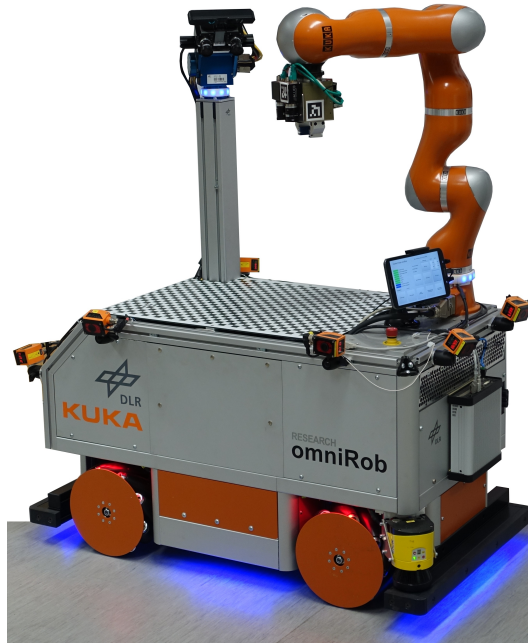
Figure 6.1: The autonomous industrial mobile manipulator AIMM
