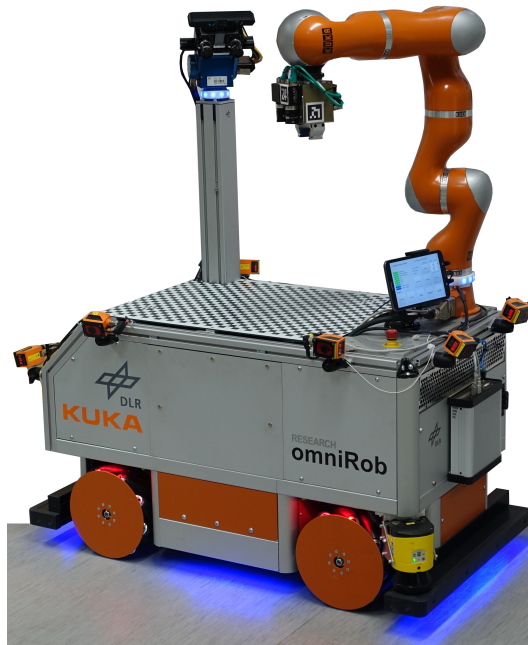
Figure A.1: The autonomous industrial mobile manipulator AIMM
