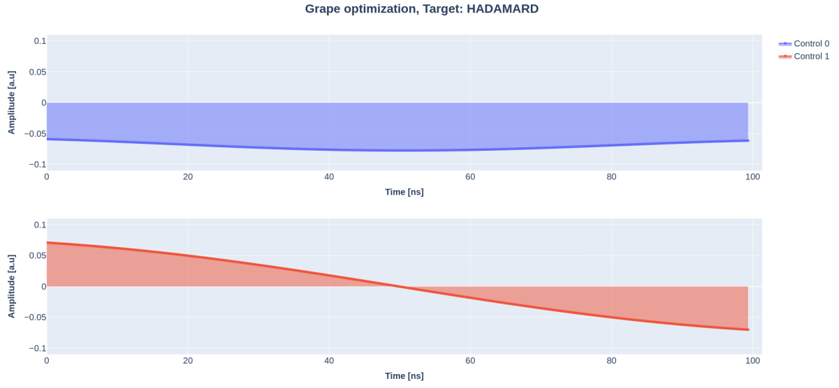
Figure 4.4.: Final control amplitudes for optimization of a Hadamard unitary with a duration of T \approx 100 ns. Control 0 corresponds to the u_1 -amplitudes driving a \sigma_X -rotation, while Control 1 represents the u_2 -amplitudes for a \sigma_Y -rotation.
