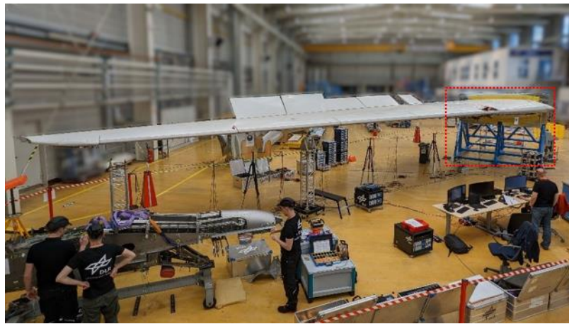
Figure 3. A320 wing attached to the wing support structure; red box: support structure [10]
