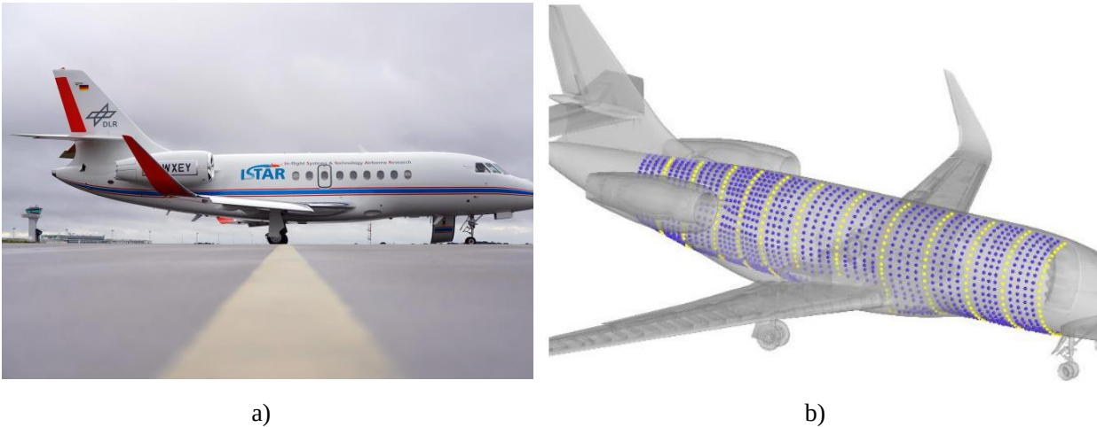
Figure 1. Dassault Falcon 2000LX [8] a) and sensor configuration for measuring the aircraft vibration [8] b)
