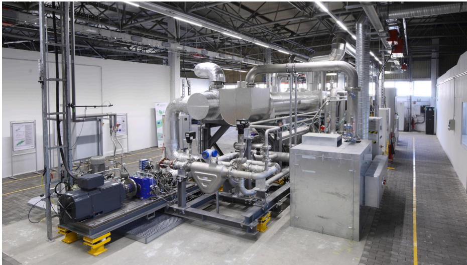
Fig. 1. Photo of the CoBra heat pump test facility.
