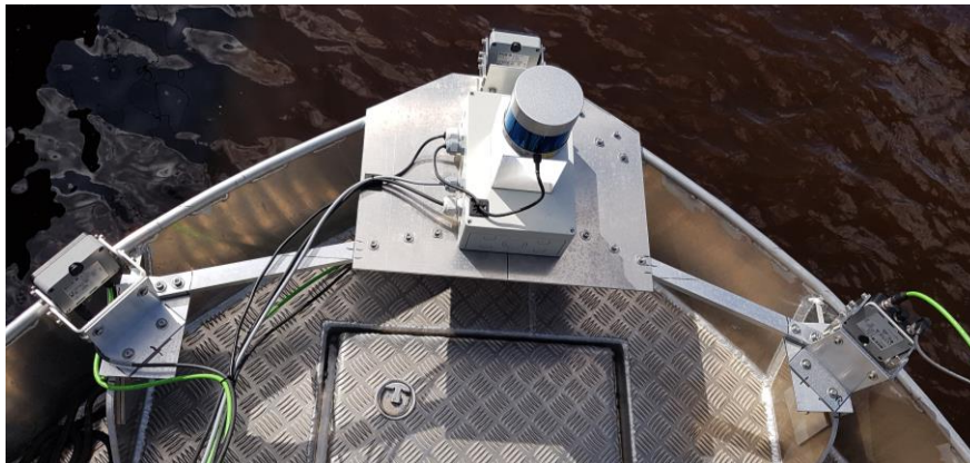
Figure 6. The platform to mount three 1D FMCW Radar sensors and a 3D LiDAR at the bow of the test vessel Sally .
