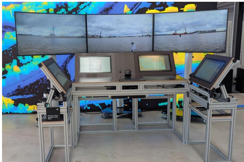
Figure 2. The Remote Operation Center setup that was built as a part of the study and used in the sea trials.
