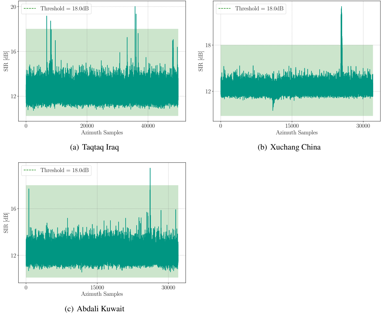
Figure 3.4: Three RFIs found that are visible in the SIR filtered profiles but that are not visible in the according processed quicklook images shown in Fig. 3.5
