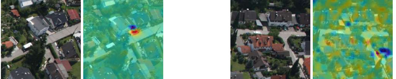
Figure 3.9: the buildings in front of the cars has affected the confidence scores of the target bounding boxes negatively ,so the model couldn't detect the vehicles
