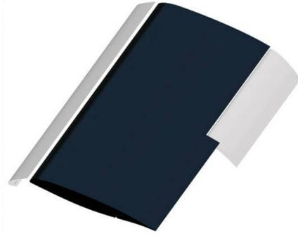
(b) 3-element high-lift model ( $s_{flap} = 0.4$  m,  $c_{flap} = 0.12$  m).
