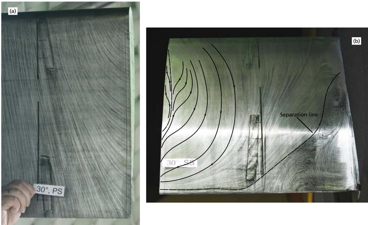
**Figure 5.4.:** Surface streaklines visualization. Approximative streaklines are sketched.  $\delta_F = 30^\circ$ . (a) Pressure side. (b) Suction side.
