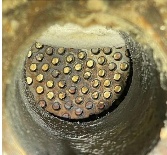
**Figure 79: Leakage of silicone at the connecting line between diaphragm and pressure sensor**
