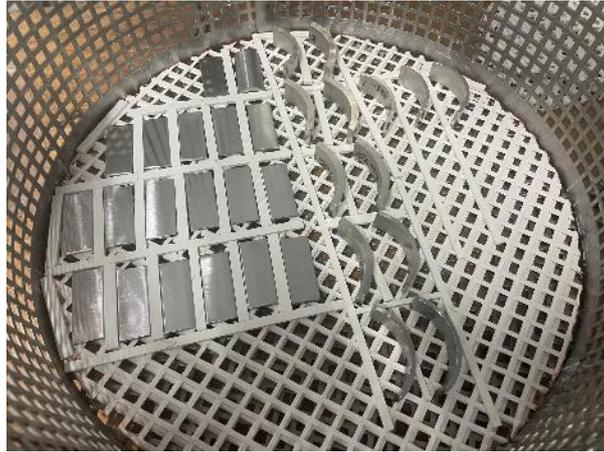
**Figure 4 Corrosion basket and placement of steel materials inside.**
