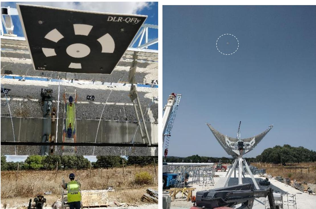
**Figure 36 – Positioning of targets (left) and execution of Qflights with DLR's drone (right)**
