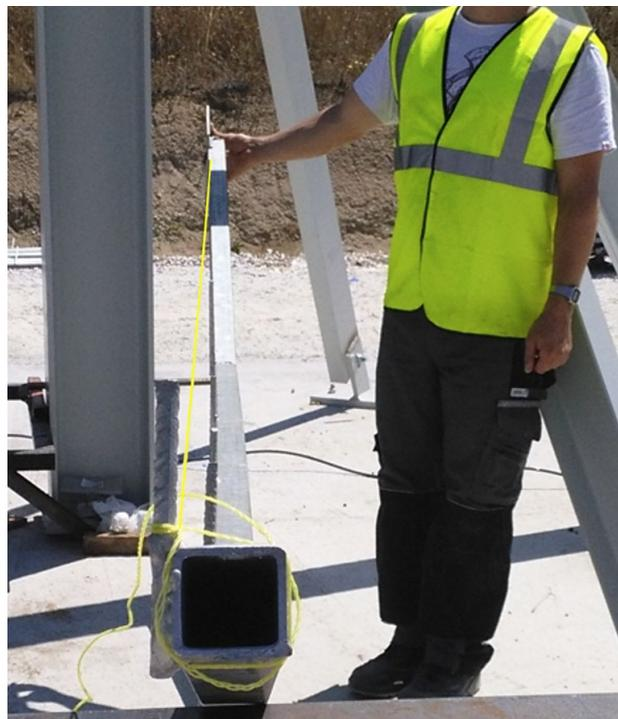
**Figure 25 – Deformation of cantilever arms due to uncompensated welding stresses**
