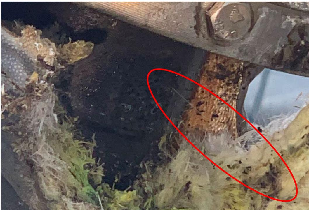
**Figure 80: Salt leakage on REPA elbow after electric arc**
