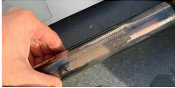
**Figure 45 Damaged plunger of feedwater pump after leakage**
