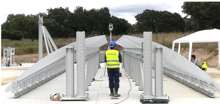
**Figure 23 – Quality control of the Assembly Jigs with Laser Tracker**
