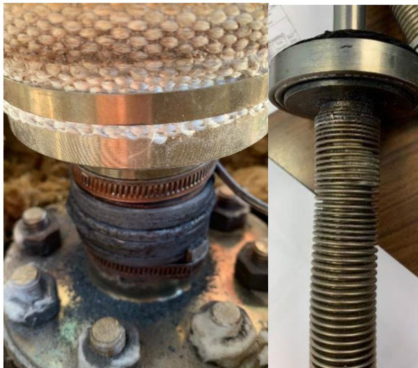
**Figure 81: Original valve bonnet heating and damages due to solid salt in gaps of the valves bellow**
