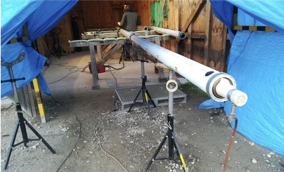
**Figure 40 – TIG-welding of the HCE triples with forming gas**
