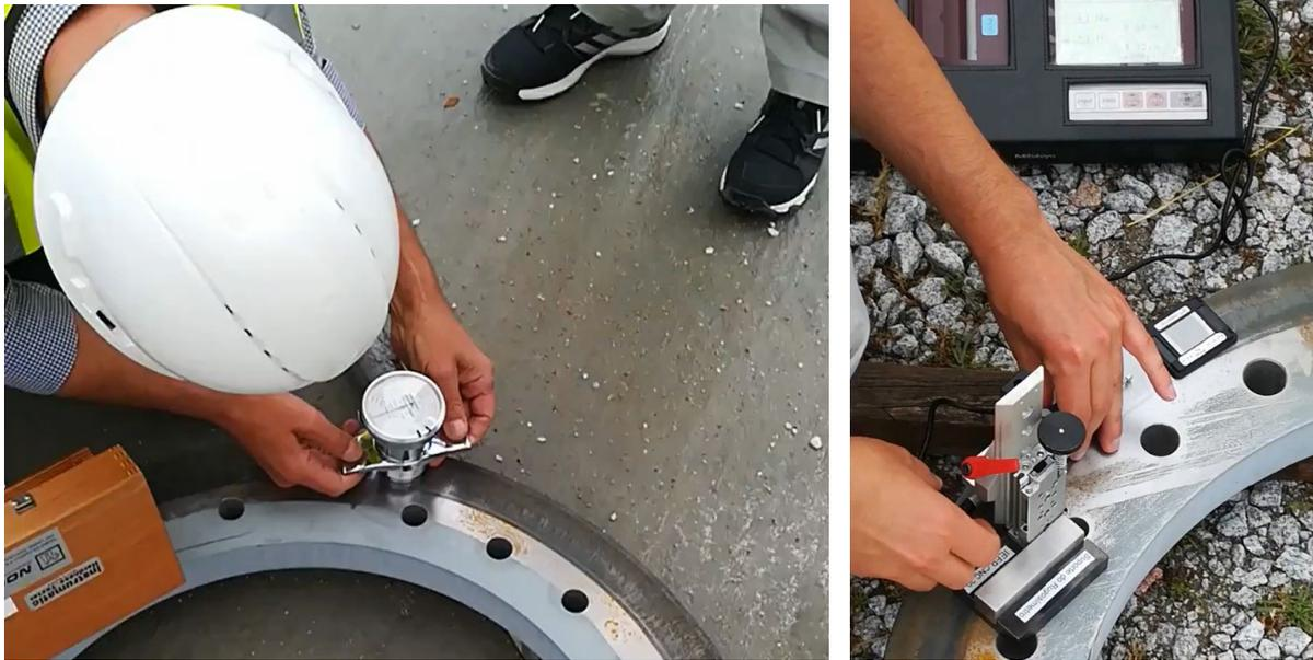
**Figure 14 - Testing of Rockwell hardness and surface roughness on bearing flanges**
