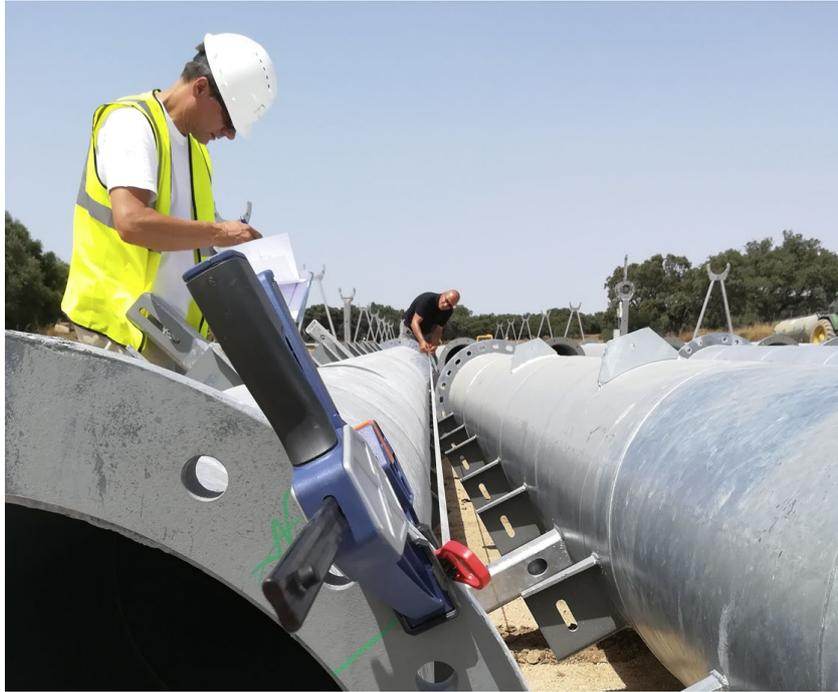
**Figure 27 – Temperature-corrected measurements of tubes for optimized TTU combinations**
