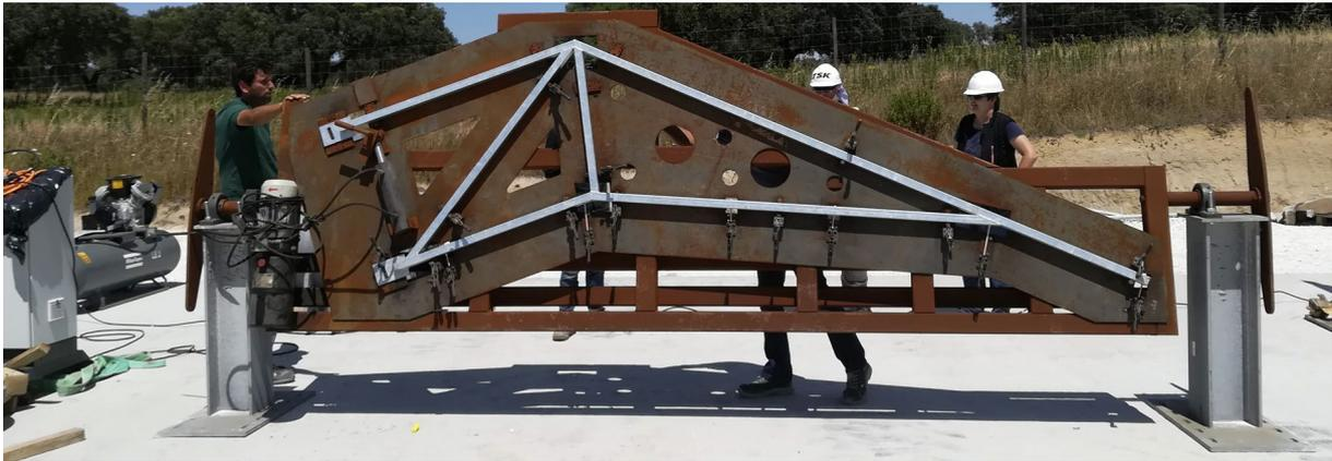
**Figure 26 - Straightening bench for cantilever rectification**
