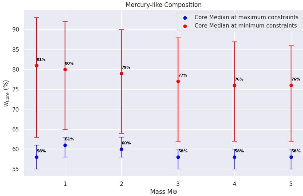
Figure 7.5: The core mass fraction vs. planetary mass plot under maximum and minimum constraints plot for planets with Mercury-like composition as a function of planetary mass. The plot shows the median core mass fraction (dots) under two different constraint conditions: minimum constraints (red) and maximum constraints (blue), with error bars indicating the range of variability for each scenario.
