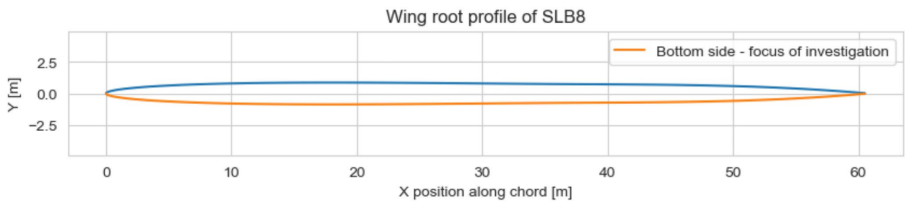
Fig. 8 Wing root profile of the Space Liner 8 vehicle (SLB8). The bottom side, the focus of this case study, is highlighted
