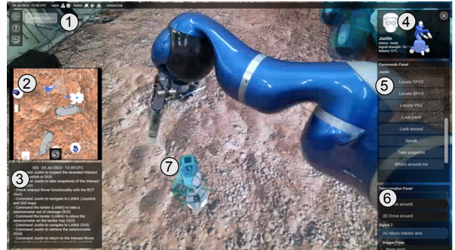
Figure 3. Screenshot of the GUI used during the Surface Avatar experiments. The parts of the GUI are: (1) view of the robot's camera, (2) a map view, (3) a messenger panel, (4) an avatar view of the robot, (5) the available task-level commands, (6) teleoperation panel, and (7) overlays marking the believed position of objects known to the robot.
