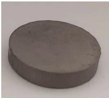
Fig. 4. Representative image of a pellet of \text{Ca}_{0.8}\text{Sr}_{0.2}\text{MnO}_3 .
