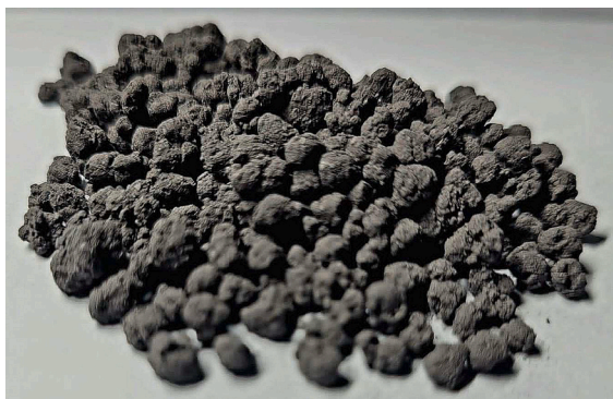
Fig. 1. Representative image of a granule of Ca_{0.8}Sr_{0.2}MnO_3 ( G CS20M0 ) with a diameter of 1.25 mm to 1.6 mm.
